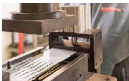
CINGHIE DENTATE IN PU SALDATE
