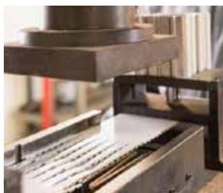
CINGHIE DENTATE IN PU SALDATE
