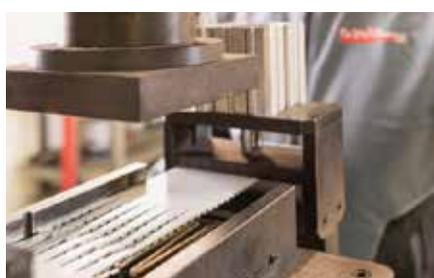
CINGHIE DENTATE IN PU SALDATE
