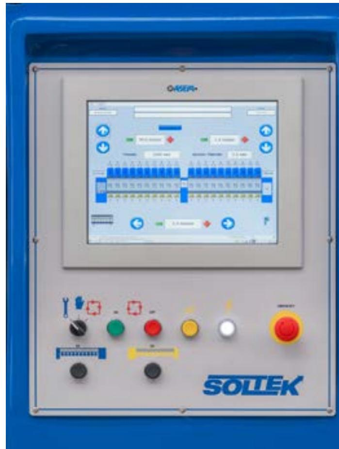
In the LS range of polishing lines, the electronics is safe and powerful. Any function can be instantly retrieved on the user-friendly control panel, where you can easily adjust any setting as you like: speed of belt, speed of beam, deceleration at the edges of the tile/slab, double polish in some places, etc. The machine has a touch-screen control panel with a colour graphic interface.
