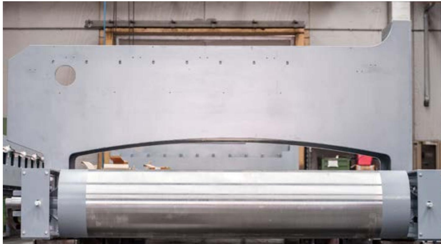
Made of metal carpentry, it is ground at the top, so the tile/slabs fit in snugly and the belt runs smoothly.
